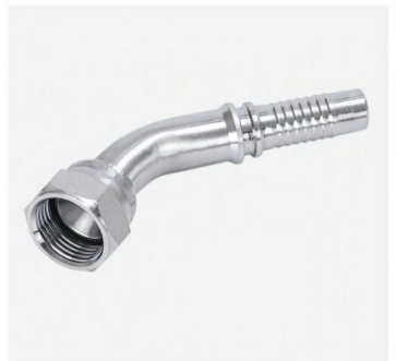
P/N:26741 45°JIC female 74° cone seat sae
