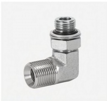
P/N:1BG9-OG 90° BSP male 60° seat/BSP male o-ring adjustable stud end
