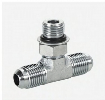
P/N:AJOJ-OG JIC male 74° cone / sae o-ring run tee
