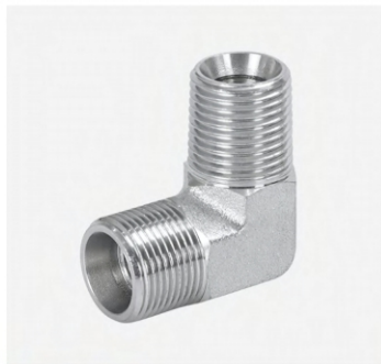
P/N:1CN9 90°NPT male /metric male 24°cone l.t
