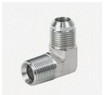
P/N:1JT9 90°elbow JIC male 74° cone/BSPT male
