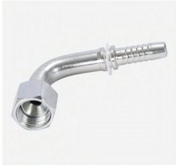
P/N:20791 90°metric female 74° cone seat
