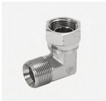
P/N:2B9 90° BSP male double use for 60° seat or bonded seal/BSP female 60° cone
