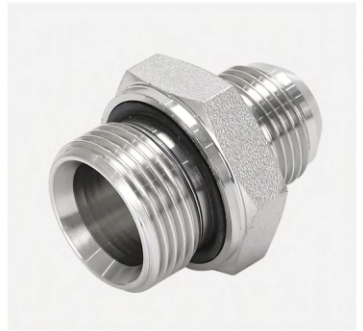
P/N:1JG JIC male 74° cone/BSP male o-ring
