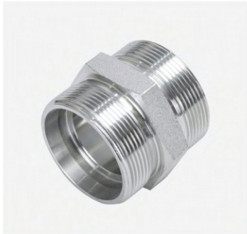
P/N:1C Metric male 24° cone L.T/BSP male with captive seal
