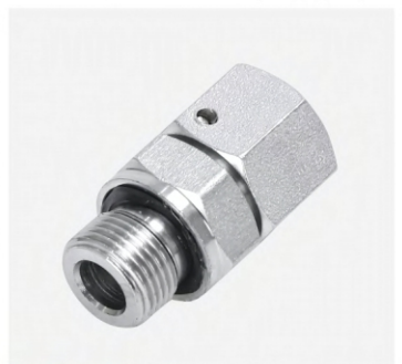
P/N:2GC BSP thread stud ends with o-ring sealing /metric female 24° cone o-ring sealing
