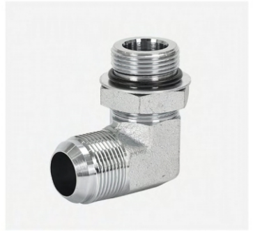
P/N:1JO9 90° elbow JIC male 74° cone / sae o-ring
