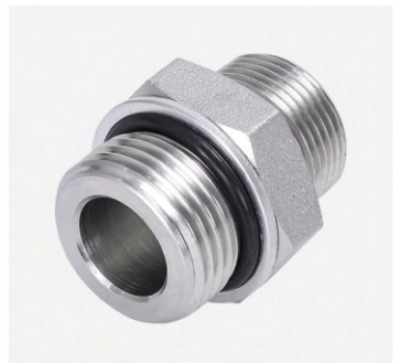
P/N:1CO UN.UNF THREAD thread stud ends with o-ring sealing
