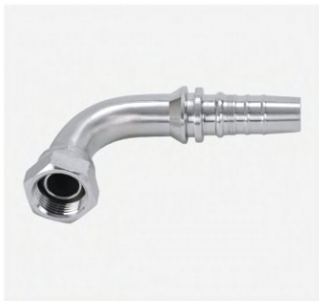
P/N:22693 90° bsp female 60° cone one piece interlock fitting
