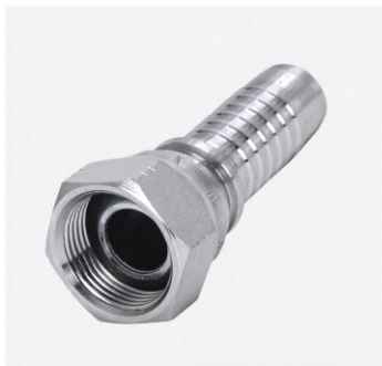
P/N:21611 NPSM female 60° cone sae
