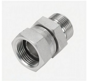
P/N:2B BSP male double use for 60° seat or bonded seal/BSP female 60° cone
