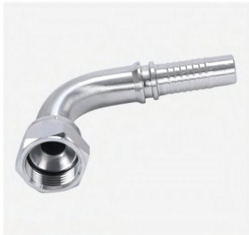
P/N:26791 90°JIC female 74° cone seat sae
