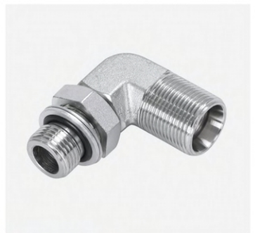
P/N:1CG9-OG 90°BSP thread adjustable stud ends with o-ring sealing
