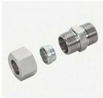
P/N:1C-RN Metric male 24° cone I.t./NPT male with cutting ring and nut
