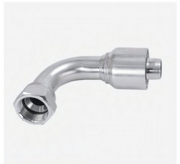
P/N:26791RW 90°JIC female 74° cone seat sae one piece
