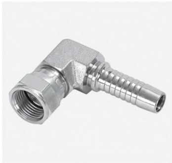
P/N:26791K 90°JIC compact female 74° cone seat sae
