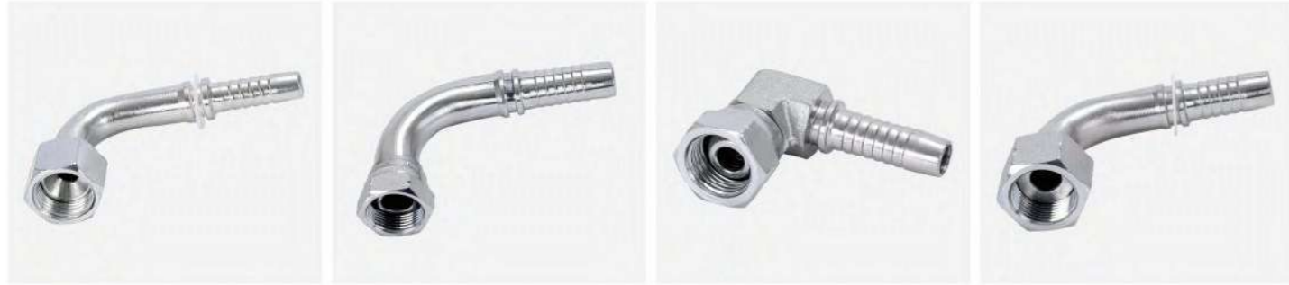
P/N:20791 90°metric female 74° cone seat P/N:22691 90°BSP female 60°cone P/N:22691K 90°BSP compact female 60° cone seat sae P/N:24291 90°ORFS female flat seat
