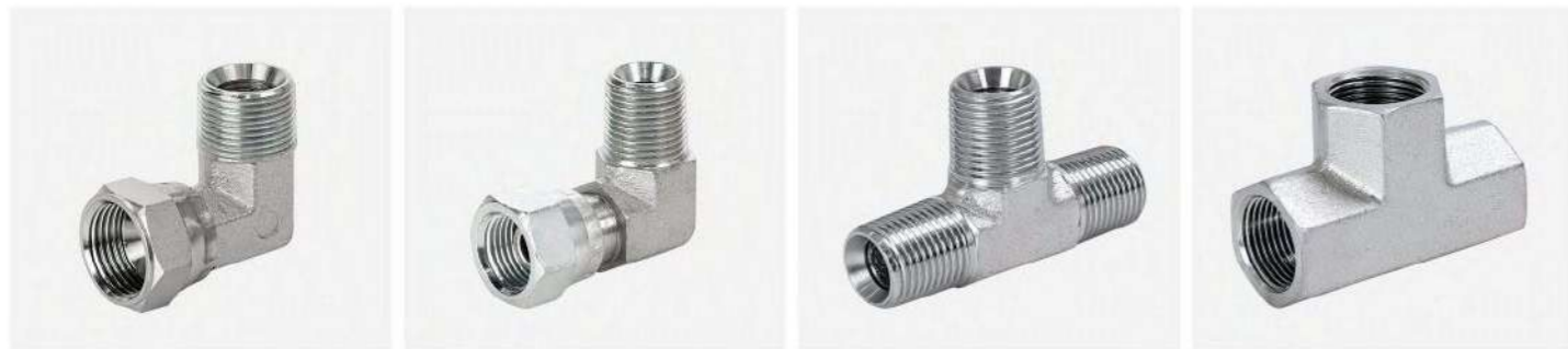
P/N:2NJ9 90° NPT male / JIC female 74° seat P/N:2NU9 90° NPT male / NPSM female 60° cone P/N:AN NPT male tee P/N:GN NPT female tee
