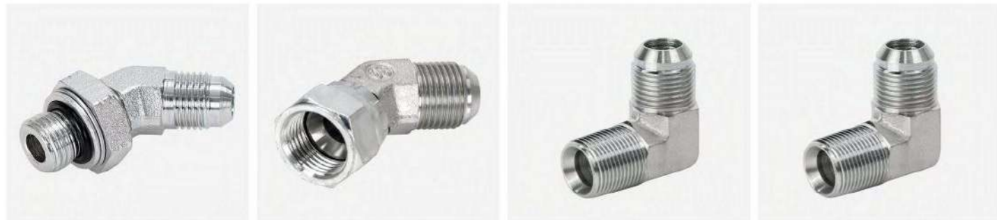
P/N:1JG4 45°elbow JIC male 74°cone /BSP male o-ring P/N:2J4 45° JIC female 74° cone/JIC male 74° cone P/N:1JN9 90°elbow JIC male 74°cone/NPT male P/N:1JT9 90°elbow JIC male 74°cone/BSPT male
